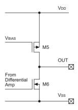
Because of the consideration for minimized power consumption, the max. output current is limited to about  $400\mu A$  for both source and sink drive. This is believed to be enough for most low power systems, however it is recommended to use the load resistor of  $>\!10k\Omega$  for normal applications. In case of heavy load driving, an external buffer stage using bipolar transistors is recommended.
